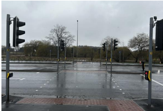
Toucan crossings over main road are useful to link sections of greenways
