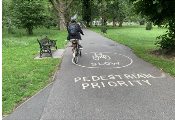
In areas with higher pedestrian and cycle flows, markings on the ground can provide helpful reminders for cyclists to use routes considerably (London Fields)
