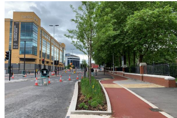
SuDS and green infrastructure should be delivered alongside active travel infrastructure wherever possible (Greater Manchester)
